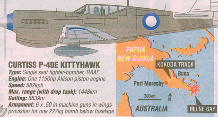
CURTISS P-40E KITTYHAWK Type: Single seat fighter-bomber, RAAF Engine: One 1150hp Allison piston engine Speed: 582kph Max. range (with drop tank): 1448km Ceiling: 8839m Armament: 6 x .50 in machine guns in wings provision for one 227kg bomb below fuselage
